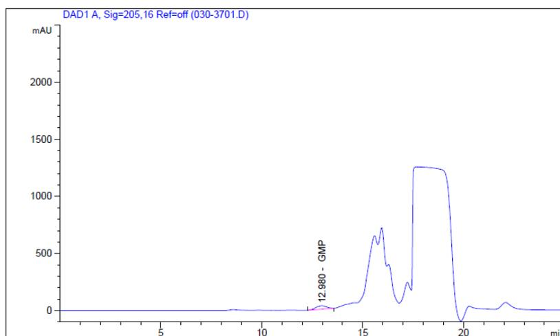
**Figure 2.** Typical chromatogram of sample determined by ultrasound precipitation method.
