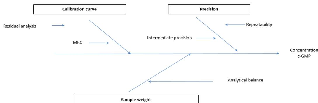
**Figure 5.** Identification of sources of uncertainty through the cause - effect diagram.
