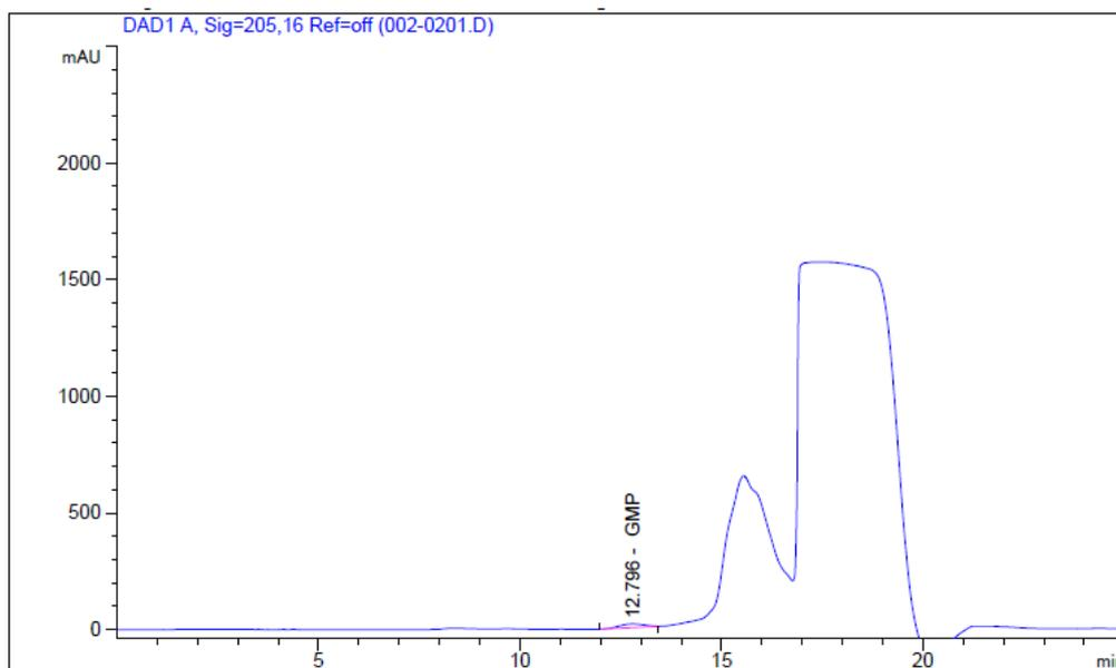
**Figure 1.** Typical chromatogram of the Lacprodan standard used in the quantification of c-GMP. The molecule of interest is marked with the response time. The signals that were not integrated correspond to trichloroacetic acid.
