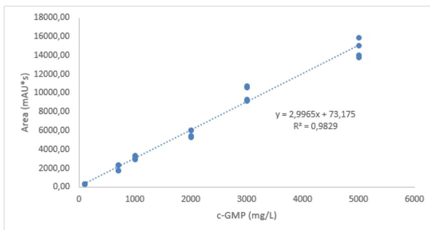
**Figure 4.** Linearity, equation of the line and correlation coefficient for high rank.
