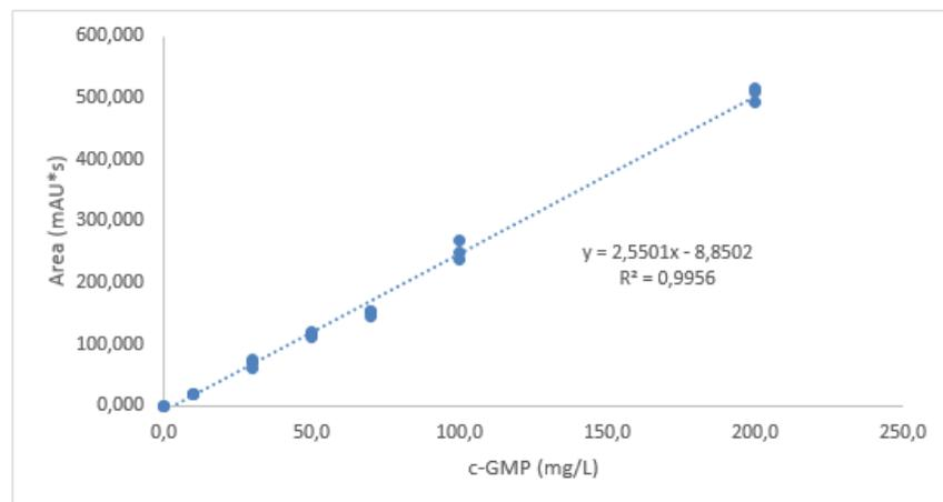
**Figure 3.** Linearity, equation of the line and correlation coefficient for low range.
